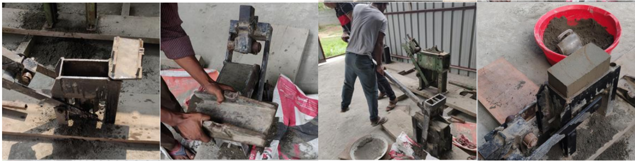
Figure 1: Compressed Stabilized Earth Block (CSEB) production [17].
